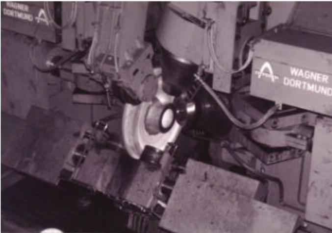
**Figure 4. A wheel is rolled in the new vertical wheel rolling mill. Note that there is no mandrel.**
