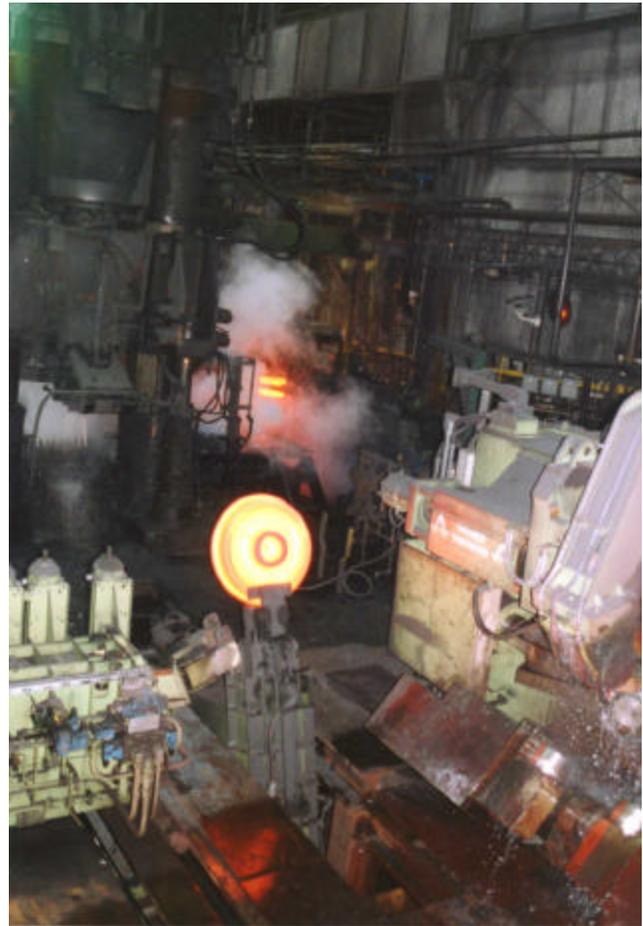
**Figure 3. A robot manipulator transferring a wheel pre-form from the 10,000 ton forging press to the rolling mill.**
