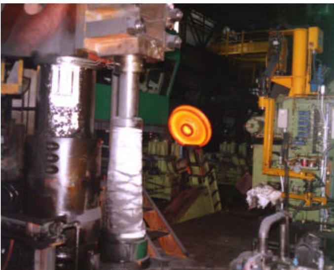
**Figure 5. A robot manipulator passes a wheel from the rolling mill to the dishing and punching press.**
