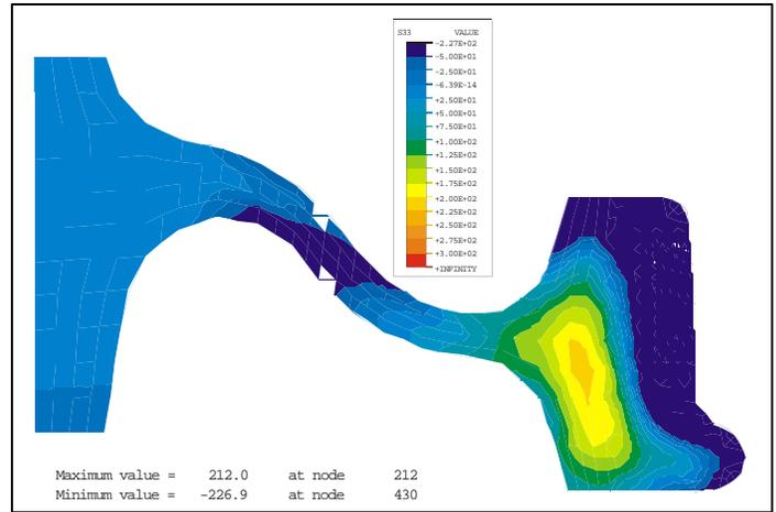
**Figure 1. Radial section hoop stress plot for a new wheel.**
