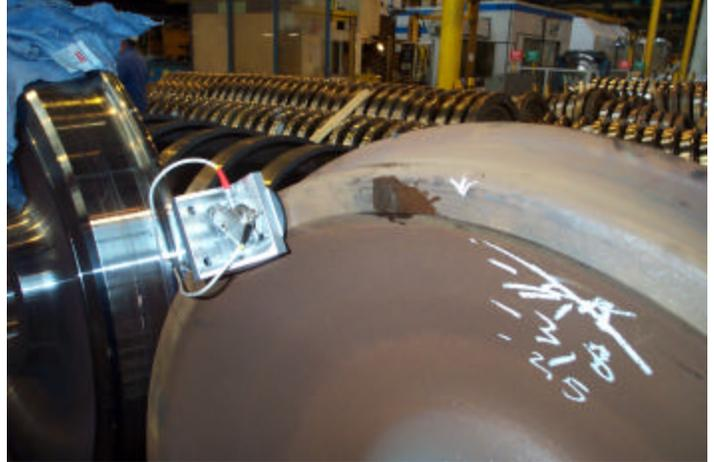
**Figure 3. The EMAT transducer on a front rim face.**
