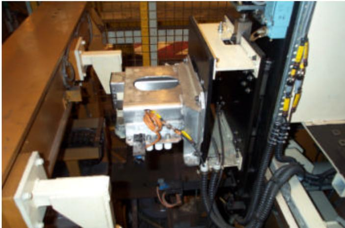
**Figure 5. Close-up view of the EMAT device used to measure wheel rim residual stresses at the Valdunes plant.**
