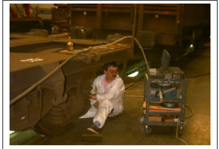
Figure 9. Residual stress measurements at SNCB.
