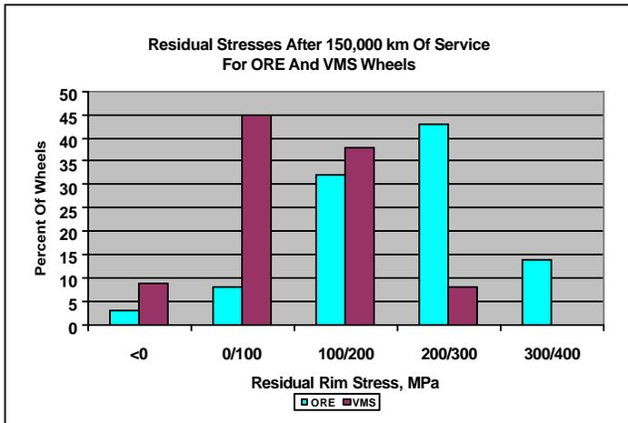
Figure 11. ORE and VMS residual stresses.
