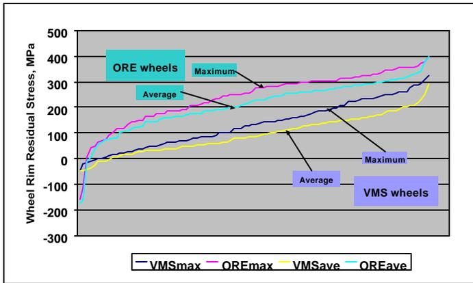
Figure 10. ORE and VMS wheel rim residual stresses.
