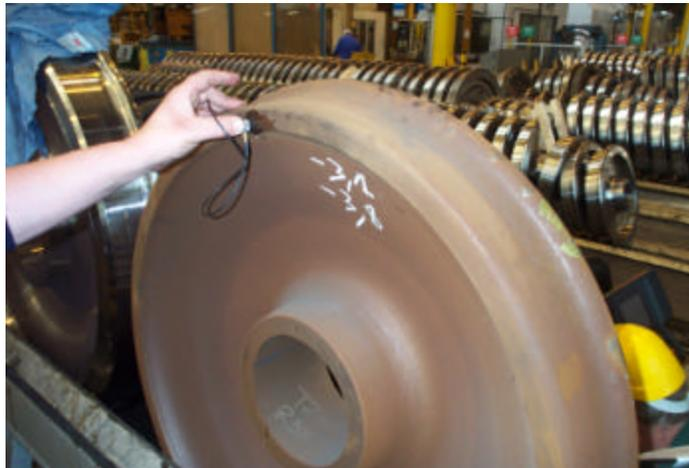
**Figure 2. Using the PET system on the front rim face.**
